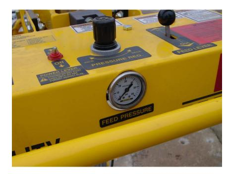
To make an adjustment on the Regulator, lift up the regulator knob, and turn it clockwise to increase the feed pressure, and turn it counter-clockwise to decrease the feed pressure.
