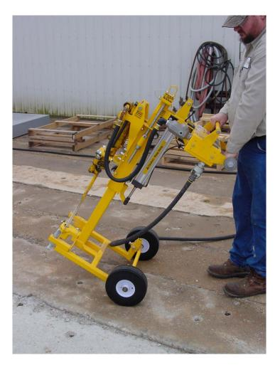
When you are finished drilling and want disconnect the air hose, first lock the carriage lock, then turn off the air supply. Before disconnecting the air hose, bleed off any air in the system by slowing turning on the power switch until all the air is released from the drill unit.
