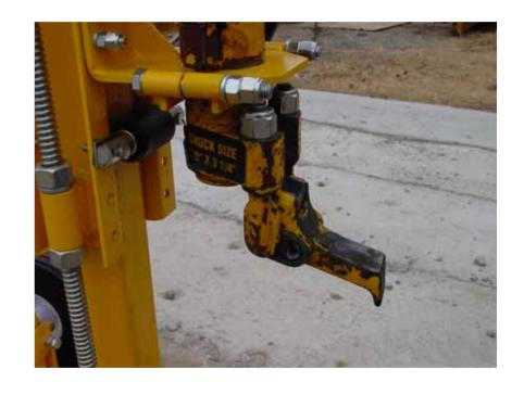
Place the bit into the chuck, close the retainer latch, and close the bit guide and tighten the swivel bolt.
