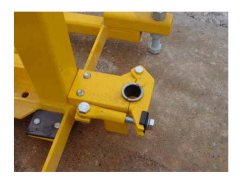
To install a drill bit, loosen the swivel bolt until you can swing it out away from the lower bit guide.
