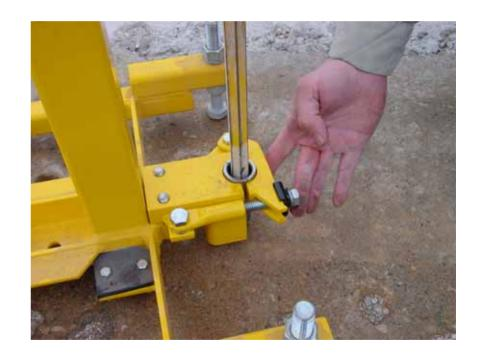
You may have to adjust the return stop rod so that the end of the bit clears the bit guide.
