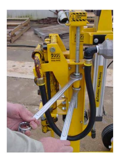
To adjust the return stop rod, loosen the stop rod nuts.
