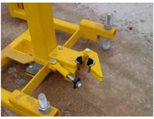
Pull down on the retainer latch on the drill motor.
