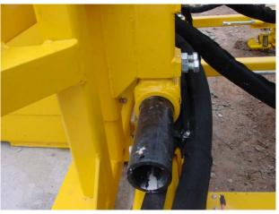
It is highly recommended that the concrete dust on the drill unit be cleaned off daily to prevent it from hardening.
