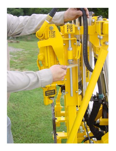
Place the proper bushing into the bit guide; one half in the upper bit guide and one half in the lower bit guide. Close bit guide, swing the swivel bolt back onto the bit guide, and tighten.
