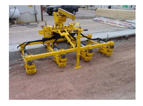
• To slide a drill system one way or the other to reach the required drill spacing, you must first loosen the 5" frame clamps on each end of each feed bar. Loosen all four ½" lock nuts on each frame clamp until you can slide the feed bar.
