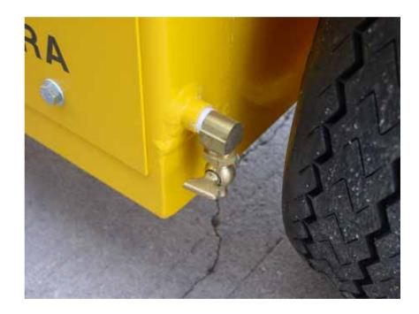
At the end of the day, use the air hose located in the oil reservoir compartment to blow off all the concrete dust from the machine.
