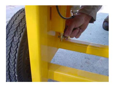
Keep all tires properly inflated (approximately 32 psi) to keep the drill unit level, and to make it easier to move.
