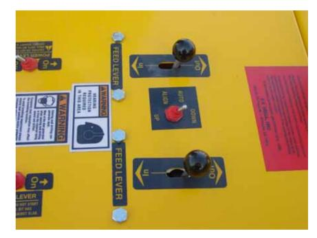
After both drills have retracted from the drilled holes, place the Auto Align Switch into the "UP" position. This will slightly raise the drills away from the concrete.
