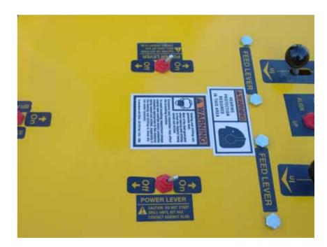
After each drill reaches its preset drill depth, it is imperative that you immediately turn that drill off. This prevents "dry-firing" (the drill is running with no pressure against the bit), which can cause extreme damage to the drill.
