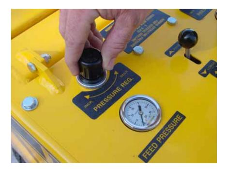
Next, place the corresponding power switch into the "ON" position. The drill will start drilling. The drill should move forward into the concrete with a slight "quiver" as it drills. If it is "bouncing", it means it does not have enough feed pressure. Lift up and slowly turn the regulator knob clockwise until the "bouncing" stops and you still have good rotation on the bit.
