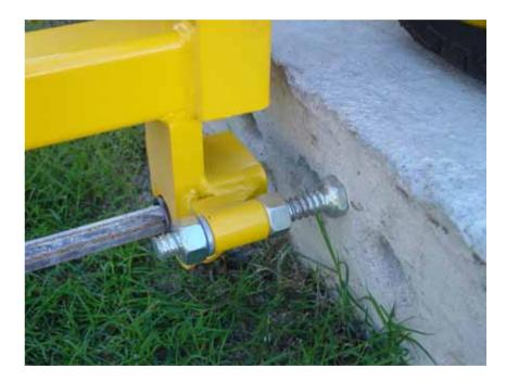
NOTE: For the drills to drill properly, and at optimum drilling speed, you may have to make some adjustments to the feed pressure on each drill. To begin with, it easier to make this adjustment one drill at a time. After making the desired adjustments to both drills, you can then start running both drills simultaneously.
