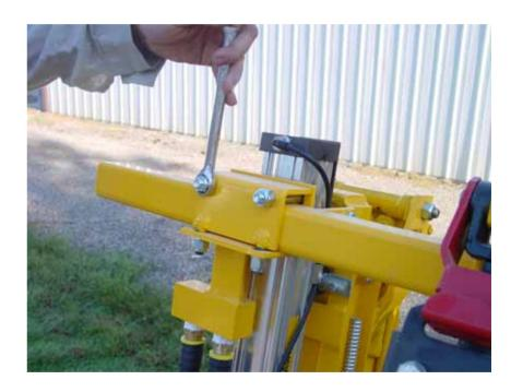
To get the proper spacing, measure from one side of the feed bar to the same place on the adjacent feed bar.
