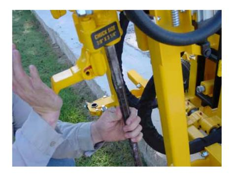
• You may have to adjust the return stop rod so that the end of the bits clears the bit guide.
