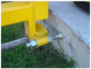
• Place the feed lever into the "IN" position. The drill will move forward until the bits contact the concrete slab.
