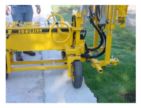
Unlock the red safety latch on the Raise & Lower Cylinders, and all of the individual carriage locks.
