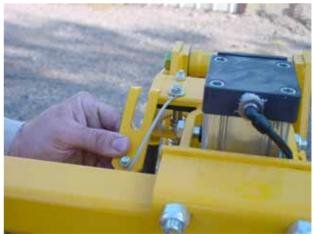
Place the "Raise & Lower" valve into the "LOWER" position. The drill systems will now lower into the horizontal position.
