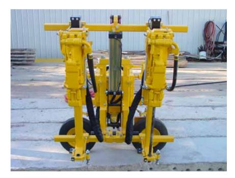
To slide a drill system one way or the other to reach the required drill spacing, you must first loosen the 5" frame clamps on each end of the feed bar. Loosen all four four <sup>1</sup>/<sub>2</sub>" lock nuts on each frame clamp until you can slide the feed bar.
