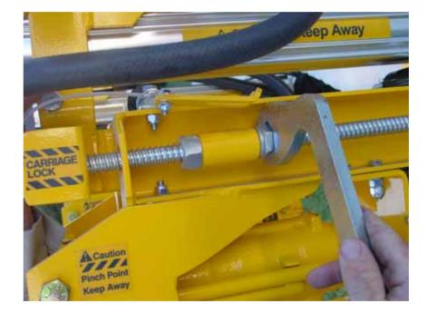
• If you are using 2-piece H-thread bits, you may also have to adjust the stop rod bolts.
