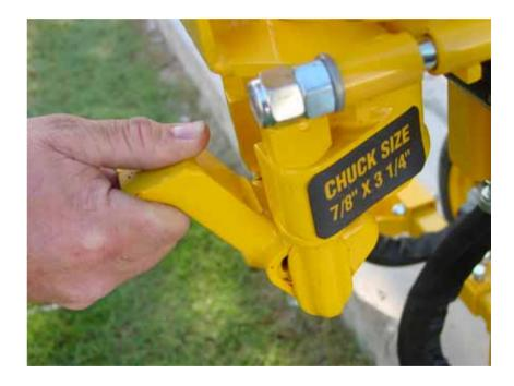
• Place the bit into the chuck and close the latch.
