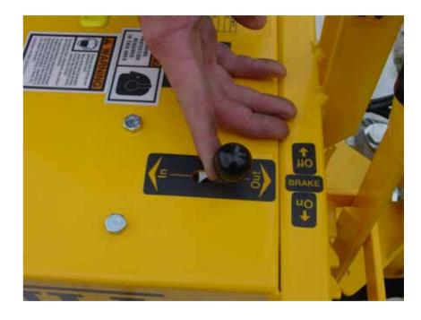
After the drill has been retracted from the drilled hole, place the Auto Align switch into the "UP" position. This will slightly raise the drill away from the concrete.
