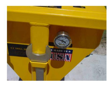
To make an adjustment on the Regulator, lift up the regulator knob, and turn it clockwise to increase the feed pressure, and turn it counter-clockwise to decrease the feed pressure. After you finish, push the knob down until it clicks.
