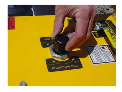
• IMPORTANT: If the drill unit is set up to drill vertical holes, the feed pressure will need to be reduced approximately 5-9 psi.
