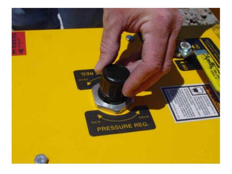
Next, turn the power lever into the "On" position. The drill will start drilling. The drill should move forward into the concrete with a slight "quiver" as it drills. If it is "bouncing", it means it does not have enough feed pressure. Lift up and slowly turn the regulator knob clockwise until the "bouncing" stops and you still have good rotation on the bit.
