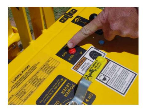
• At this point, the two guide plates/guide wheels should both be touching the face of the concrete. If one or both are not touching the concrete, the drill unit is too close to the edge of the slab, and you will need to reposition a little farther away from the edge.
