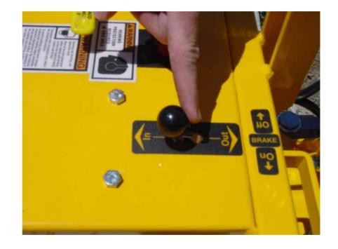
After the bit makes contact with the concrete, place the power lever into the "ON" position. The drill will start drilling.
