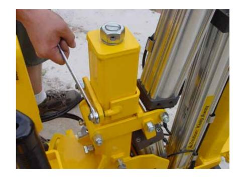
You may have to adjust the nuts on the Auto Align cylinder to bring the drill system in the exact vertical position.
