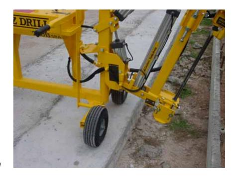
Unlock the Safety Latch and the Carriage Lock.
