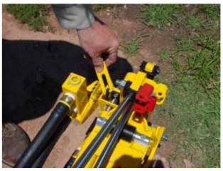
Place the Raise & Lower valve into the "Lower" position.
