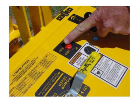
When you are finished drilling for the day, and want to move the drill unit away from the edge of the slab, place the Raise and Lower Valve into the "RAISE" position.
