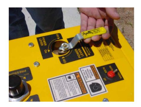
After the drill reaches its preset drill depth, it is imperative that you immediately turn the drill off. This prevents "dry-firing" (the drill is running with no pressure against the bit), which can cause extreme damage to the drill.
