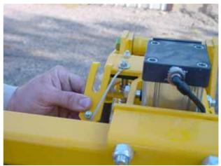
• You can store the lock pin in the holes in bracket next to the red safety latch.
