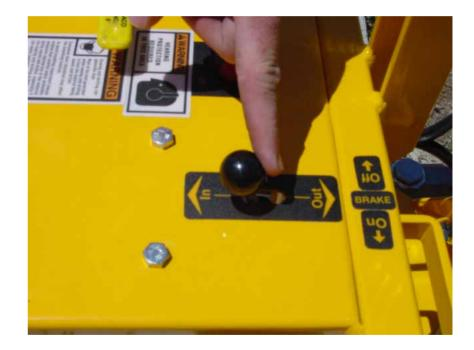
Measure the distance from the head of the stop rod to the rubber stop pad. If this is not the required drill distance, loosen the stop rod nuts and move the stop rod the desired distance from the stop pad. Re-tighten the stop rod nuts.
