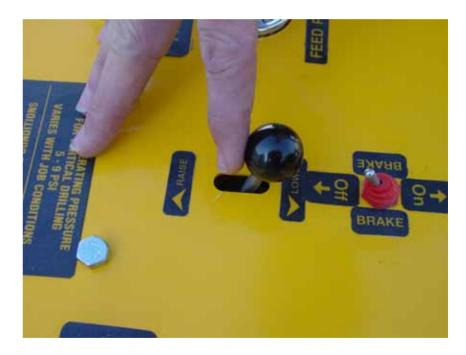
Place the "Auto-Align" switch to the "DOWN" position.
