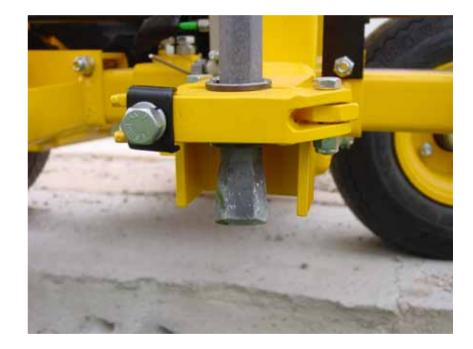
To adjust the stop rods, loosen the stop rod nuts. Move the stop rod in the direction needed to the required location and re-tighten the nuts.
