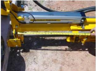
• Place the Feed Lever into the "IN" position. The drill will move forward until the bit contacts the concrete slab.
