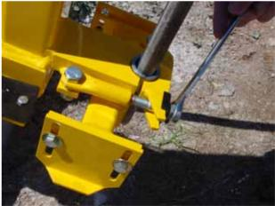
• You may have to adjust the return stop rod so that the end of the bits clears the bit guide.
