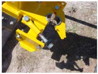
• Open the retainer latch on the drill motor.
