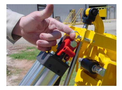
Place the "Raise & Lower" valve into the "LOWER" position. The drill system will now lower into the horizontal position.
