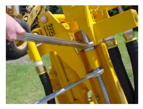
If you are using 2-piece Hthread bits, you may also have to adjust the guide plates.
