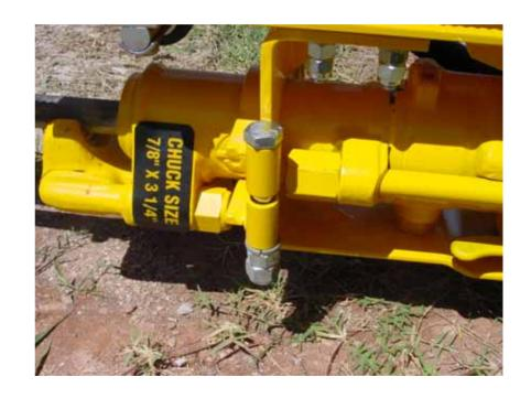
Check all nuts and bolts around the carriage assembly daily, and especially the stop rods. Tighten as needed.
