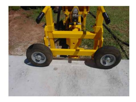
It is highly recommended that the concrete dust on the drill unit be cleaned off daily to prevent it from getting wet and hardening.
