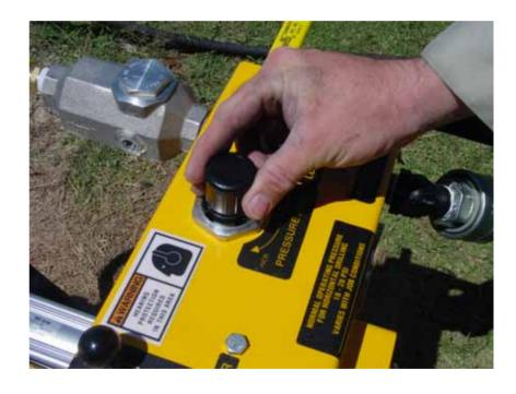
Turn the power lever to the "ON" position. The drill will start drilling. The drill should move forward into the concrete with a slight "quiver" as it drills. If it is "bouncing", it means it does not have enough feed pressure. Lift up and slowly turn the regulator knob clockwise until the "bouncing" stops and you still have good rotation on the bit.
