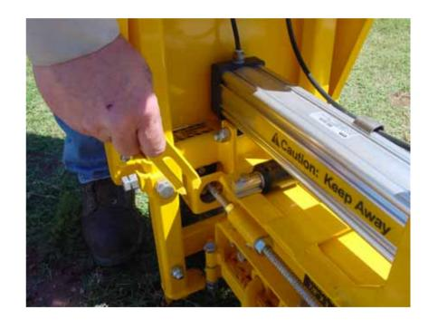
To make the feed pressure adjustment to the drill, place the Feed Control Valve into the "In" position.
