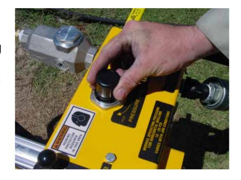
IMPORTANT: If a Vertical Conversion Kit is ever installed so that the Model 210B can drill vertical holes, the feed pressure will need to be reduced approximately 5-9 psi.
