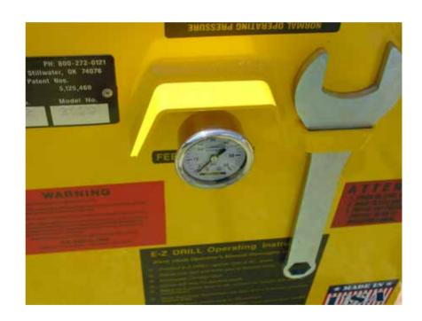
To make an adjustment on the Regulator, lift up the regulator knob, and turn it clockwise to increase the feed pressure, and turn it counter-clockwise to decrease the feed pressure.
