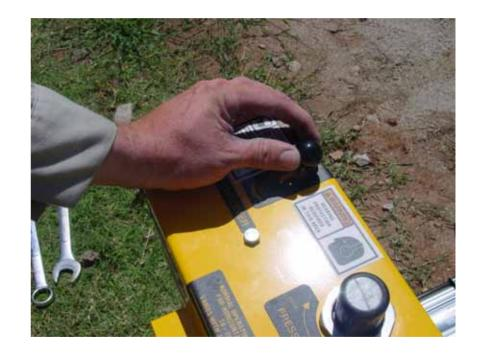
After the bits make contact with the concrete, place the power valve into the "ON" position.
