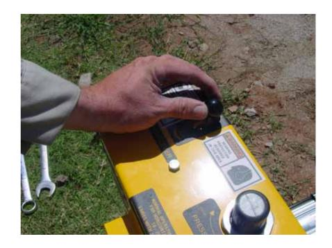
Roll the drill unit sideways to the next hole location. If you are using the optional Hole Spacing Guide, roll the unit until the Hole Spacing Guide is pointing to the last holed drilled. When the unit is in position for the next hole, repeat previous instructions.
