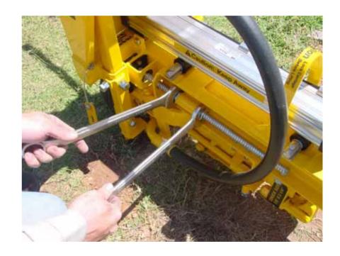
If you are using a 2-piece Hthread bit, you may also have to adjust the guide wheels by loosening the guide wheel bolt and sliding the guide wheel forward.
