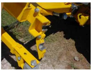
Open the retainer latch on the drill motor.
