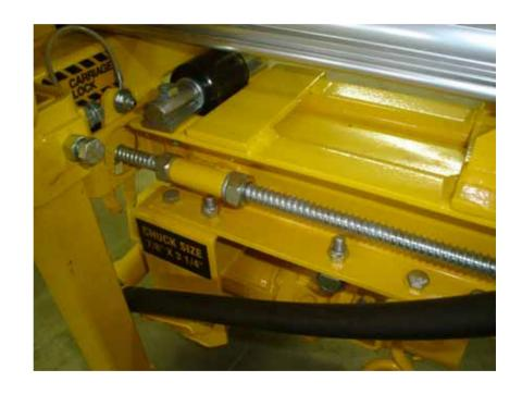
Adjust the return stop rod so that the bit will not retract so far that the bit wedges in the bit guide, but far enough that it will retract the end of the bit out of the drilled hole.
