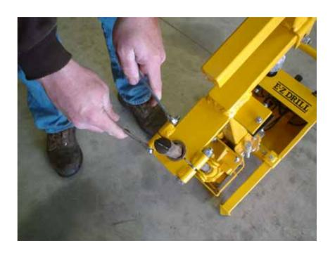
To adjust the return stop rod, loosen the stop rod nuts.
