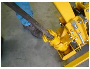
Tighten the two bolts on the bit guide. You may have to adjust the return stop rod so that the end of the bit clears the bit guide.
