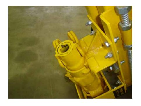
To install a drill bit, loosen the bolts on the lower bit guide using 9/16" wrenches until you can slide the end of the bit through the bit guide.
