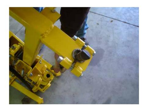
Place the bit into the chuck and close the retainer latch.
