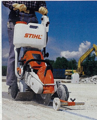
Most cut-off machines come with features and accessories, such as water tanks that promote wet cutting capabilities.
