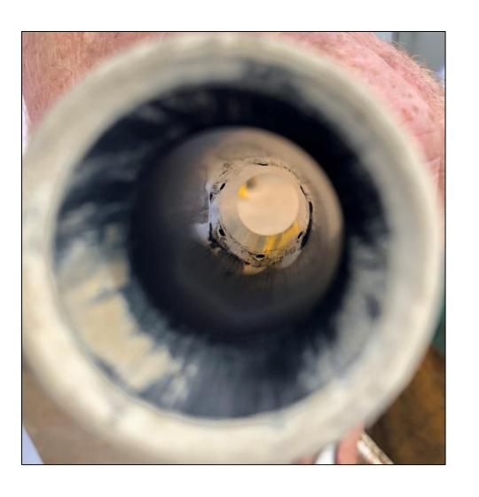
Once you have cleaned the inside of the venturi cylinder install it back on the canister. Once secure, tighten the screw clamps. After the screw clamps are tight, replace the front plate and secure with bolts.
