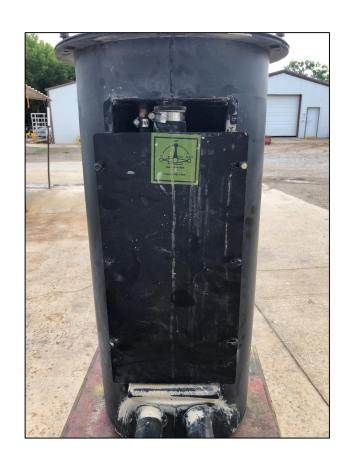
Remove the 6 bolts that hold the front plate on to the canister so the venturi is exposed.
