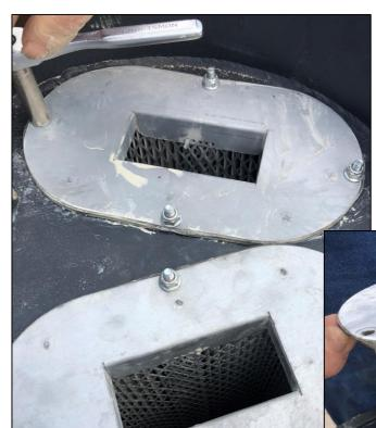
Remove the nuts from the top of the filters and then pull filters straight up to remove them from canister.
