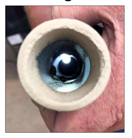
Once the venturi is removed you will need to inspect the inside, looking for buildups of dust. Take a flathead screwdriver and run it along the interior walls to remove buildups. Once large pieces are removed use a round brush and work it back and forth to clean out the rest of the dust.
